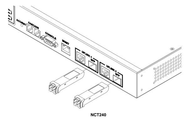
Figure 4-5. Inserting an SFP Transceiver into the Slot
